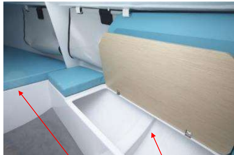
Insubmersibility foam under front sleeping. 1.60 m 3 /2 yd cubed
