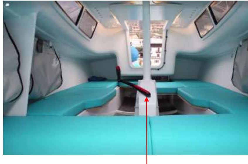
Space to lift the keel. Tip: A specific end-piece has been designed to hook up a drill to motorize keel manoeuvres
